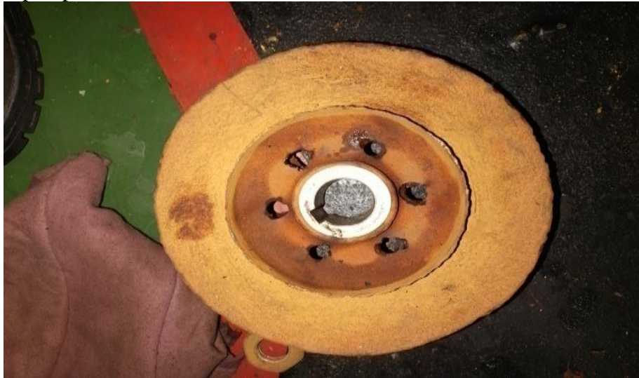
Figure 3. dirty seawater pump impeller.
